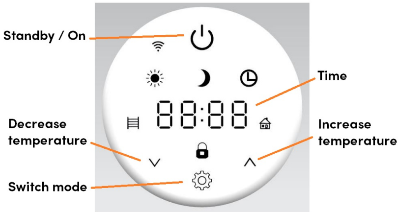
Figure 8 | Control dial display
